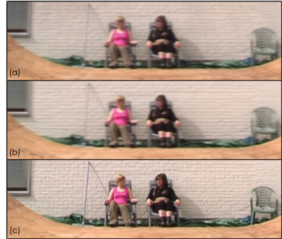
Figure 6: Comparison of (a) temporal mean filtering, (b) temporal median filtering, and (c) our background estimation algorithm.
